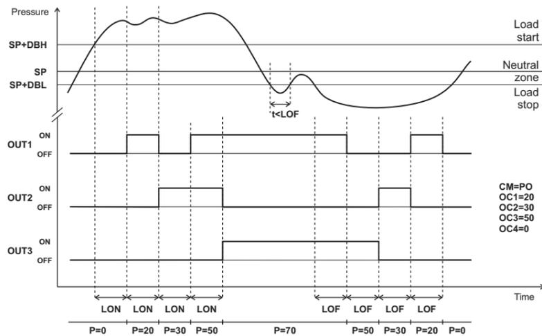
Fig.4 Control by optimisation of the available power
